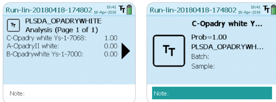
Figure 4. TruTools PLSDA model run on a TruScan RM shows definitive results.
